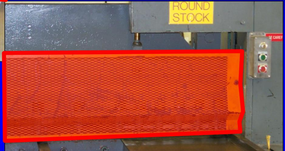
The shear guard should be set as low as possible, allowing only enough room for sheet stock. Its purpose is to keep your hands away from the point of operation, and must NEVER be removed.
