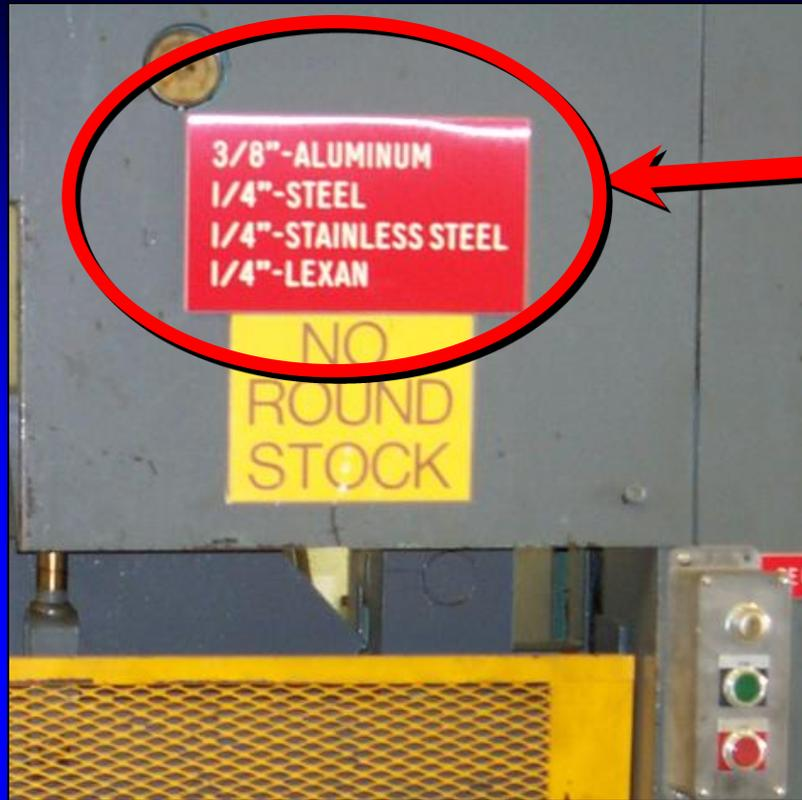
Before cutting sheet metal with a shear, ensure that it is rated to cut the gauge of sheet metal you're working with. The gauge rating is generally marked on the machine.
