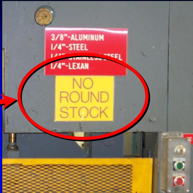
Remember that the shear is for sheet metal only. They are not built to cut round stock, and present serious hazards if anything other than sheet metal is used.
